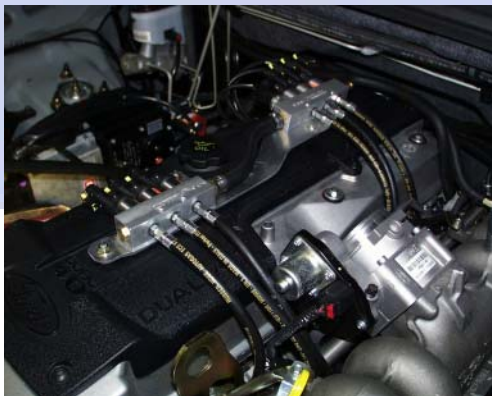
Left: VSI system installation is neat and operates flawlessly even in hot/cold start situations
